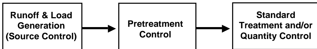
Figure 3-6 Generalized Stormwater Treatment Train
